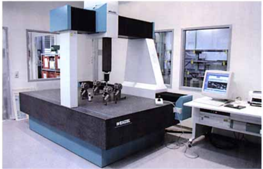
Precise dimensional scanning of mixhead housings with the 3-coordinate measuring machine.
