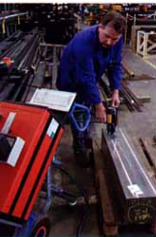
Tool steels are examined by spectral analysis.
