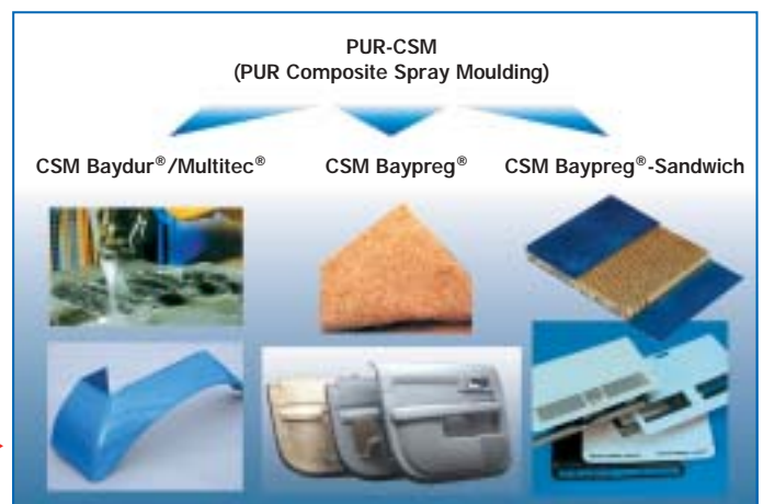
Fig. 1: PUR-CSM technology – process variants
