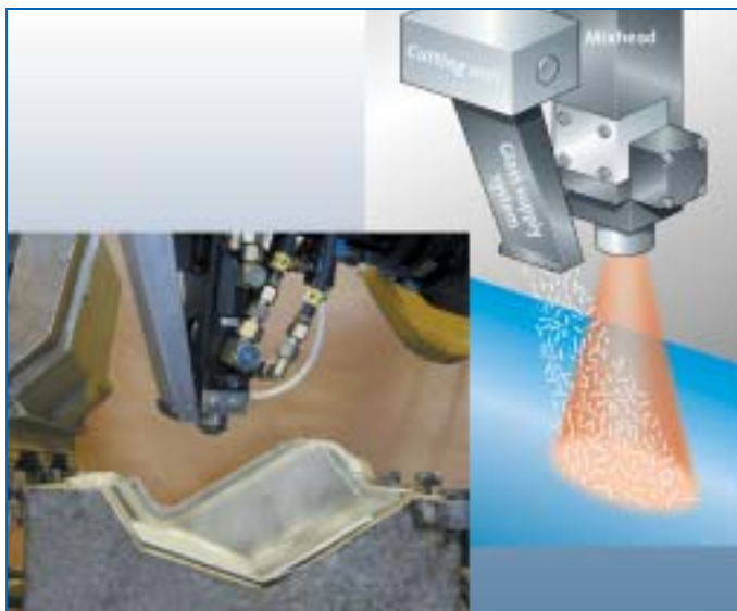
◀ Fig. 9: Long fibre spray application with PUR-CSM
