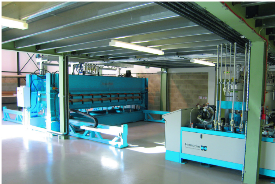
Efficient production of PU sandwich panels: Hennecke metering technology and discontinuous presses made by AutoRIM
