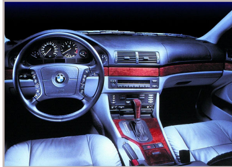
BMW cockpit featuring components with ClearRIM wood veneer surface
