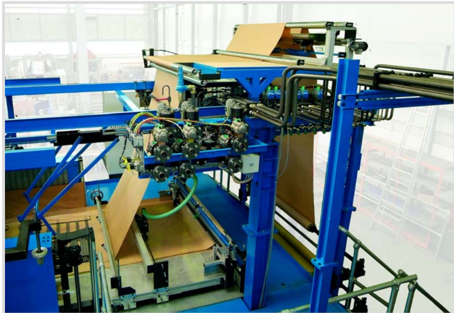
Mixer unit with liquid laydown Photo: Hennecke GmbH
