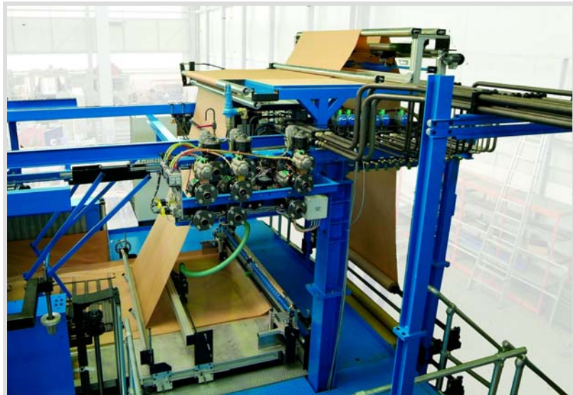
Mixer unit with liquid laydown
