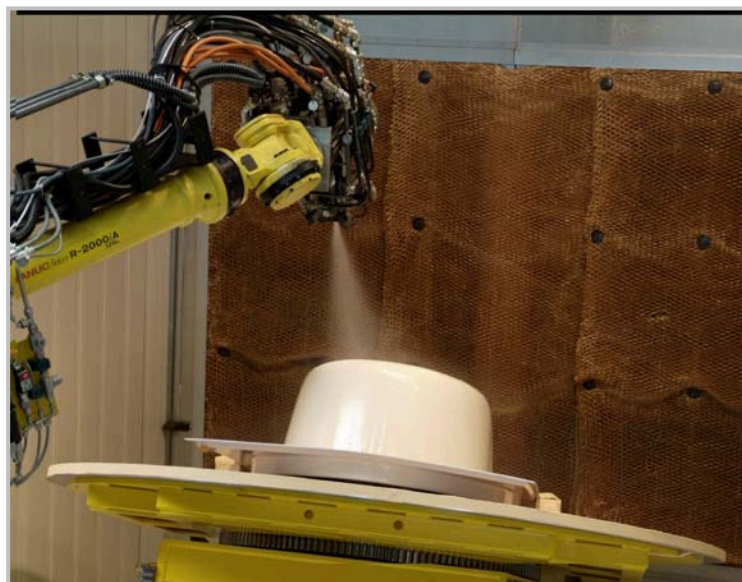
PUR-CSM spraying process Photo: Hennecke GmbH
