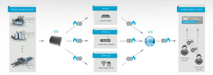
The necessary technology based on the Process Data Acquisition (PDA) software is already installed in each Hennecke plant with PC terminal. For machines and systems in which only PLC automation is being used, the data connection for remote service is established over a Remote Service Router (RSR)\*. Both solutions impose **minimum requirements on your firewall** because only two communication ports are used in the entire communication process:
