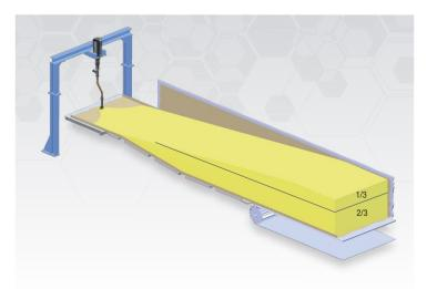
The fall plate section is ideally configured so that the feed table is at a relatively high position to the conveyor, corresponding to approx. two thirds of the foam height. The conveyor speed is selected to ensure that the foam at the end of the fall plate reaches its full height.
