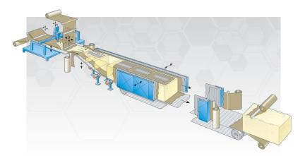
The air shutter must be positioned so that it runs crossways to the foaming direction and parallel to the laydown plate. This creates an even gap between the air shutter and the feed table. In the direction of foaming, the air shutter must be positioned 300 mm behind the mixer outlet.
