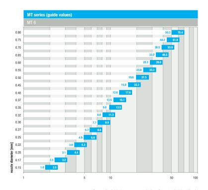
Output of individual component ccm/s (for a flow rate of 100 - 140 m/s)
