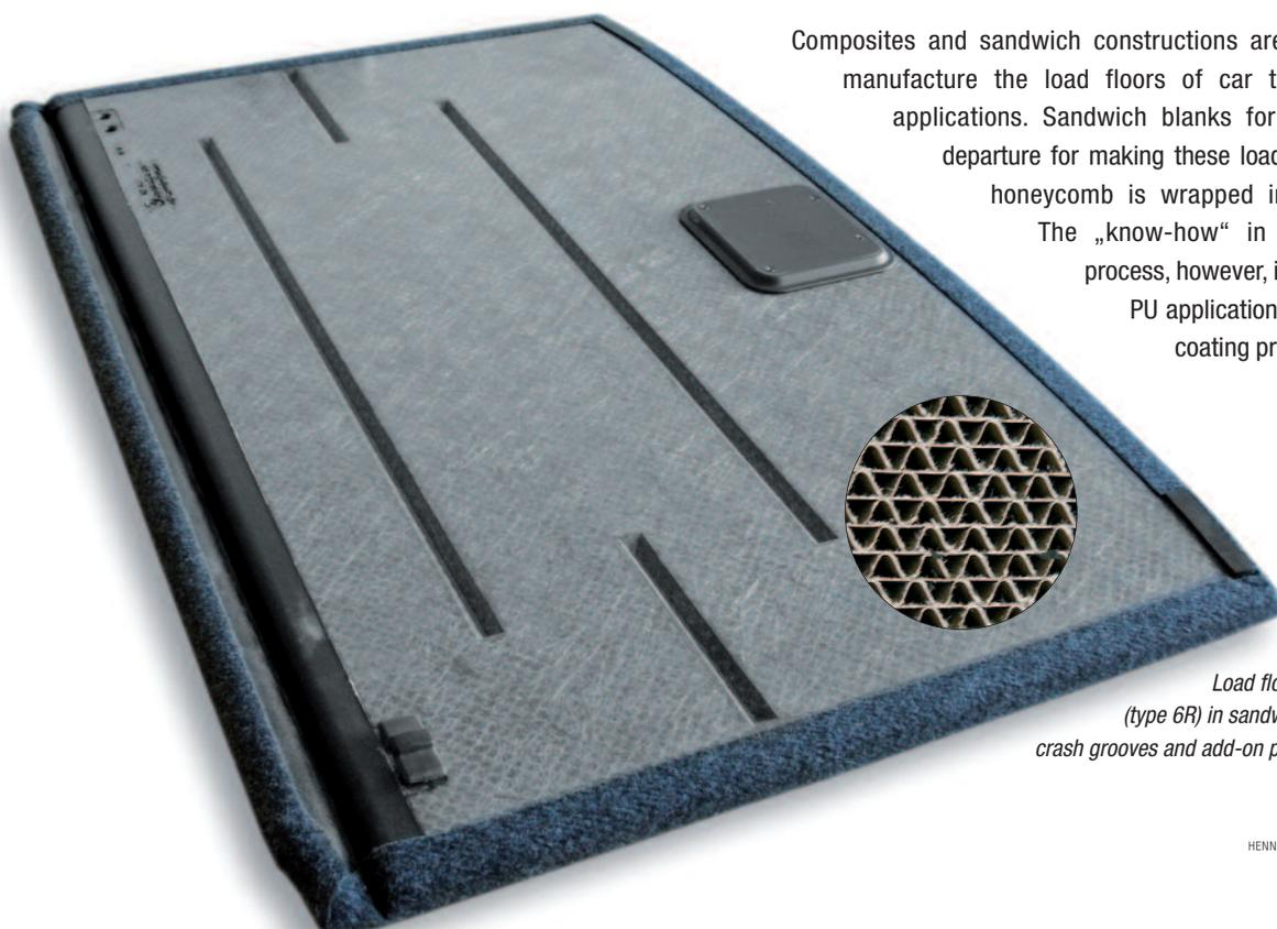
*Load floor of the VW POLO (type 6R) in sandwich design with crash grooves and add-on parts*
