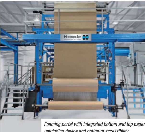
*Foaming portal with integrated bottom and top paper unwinding device and optimum accessibility*
