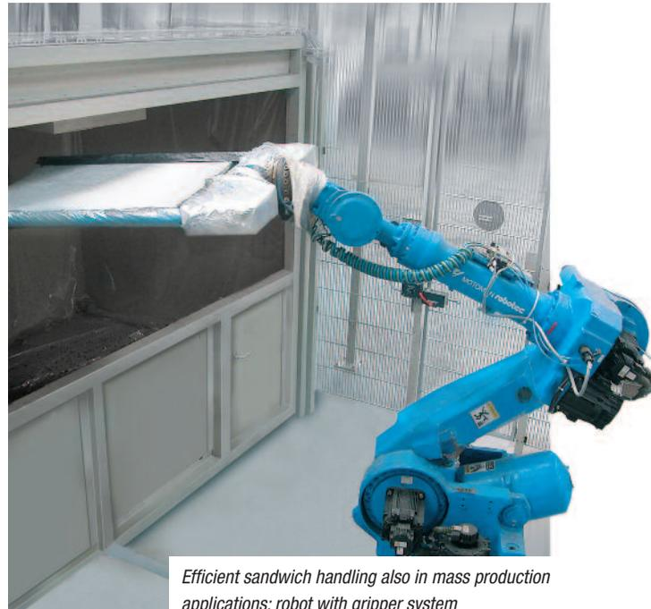
*Efficient sandwich handling also in mass production applications: robot with gripper system*
