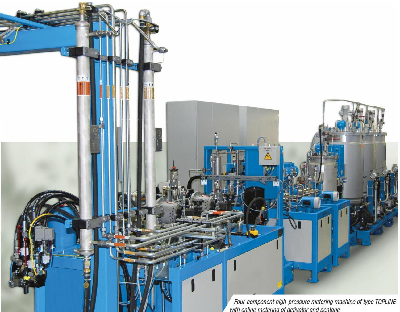
*Four-component high-pressure metering machine of type TOPLINE with online metering of activator and pentane*
