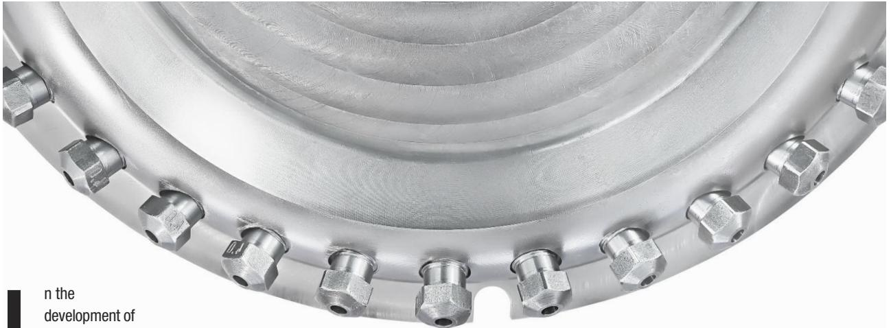
In the development of the new discharge system, the focus was placed on the way in which the liquid raw material mixture is dispensed within the production line. This requires a uniform distribution over the entire foaming width combined with a foaming reaction that starts precisely at the same time. Discharge systems used up to now have either used several mixheads or various different mechanical distribution systems to achieve the best possible combination of these two properties.
