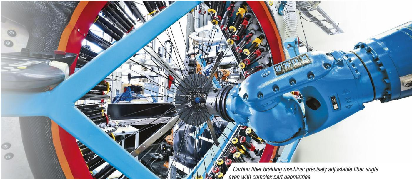
Carbon fiber braiding machine: precisely adjustable fiber angle even with complex part geometries
