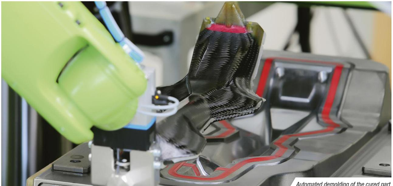
*Automated demolding of the cured part*
