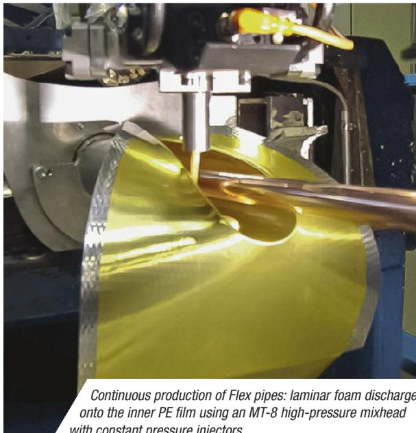
*Continuous production of Flex pipes: laminar foam discharge onto the inner PE film using an MT-8 high-pressure mixhead with constant pressure injectors*
