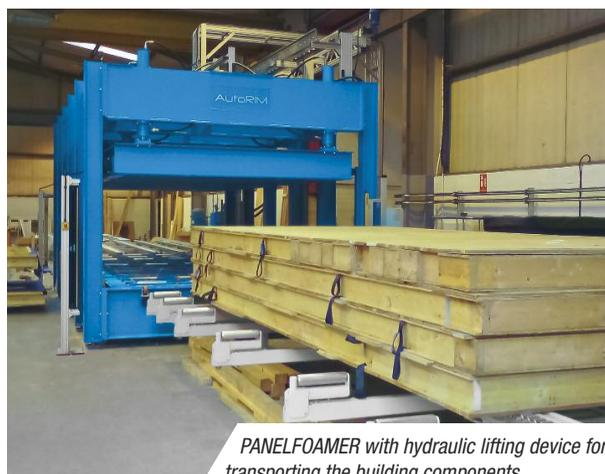
*PANELFOAMER with hydraulic lifting device for transporting the building components*
