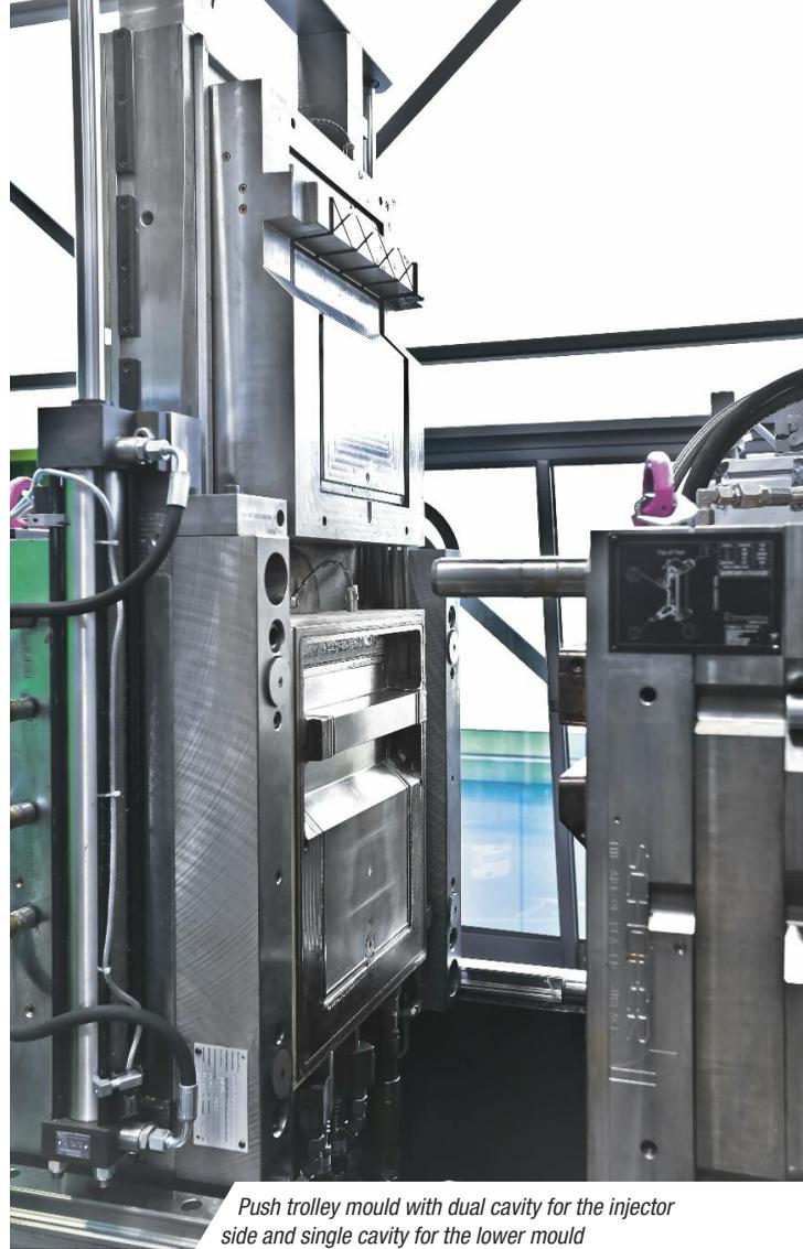
*Push trolley mould with dual cavity for the injector side and single cavity for the lower mould*
