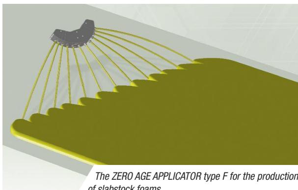
*The ZERO AGE APPLICATOR type F for the production of slabstock foams*
