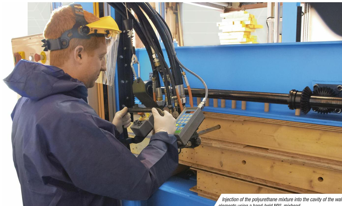
*Injection of the polyurethane mixture into the cavity of the wall elements using a hand-held MXL mixhead*
