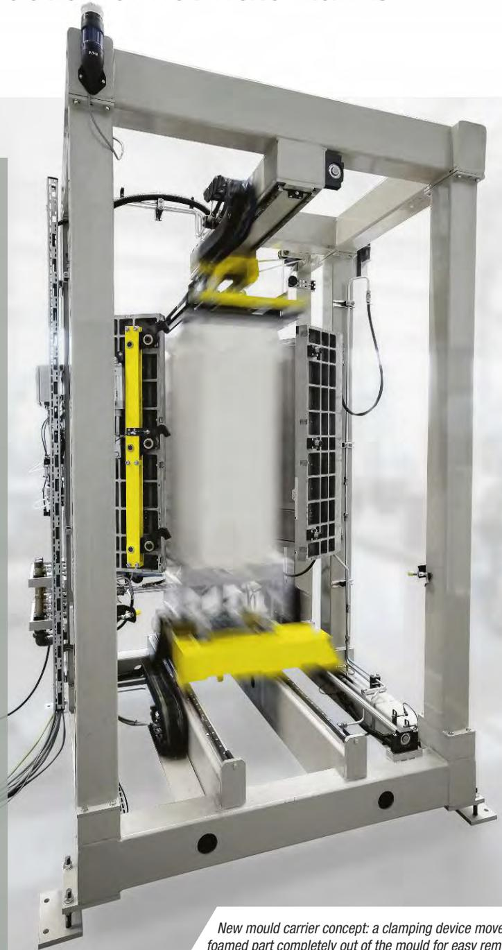
*New mould carrier concept: a clamping device moves the foamed part completely out of the mould for easy removal*
