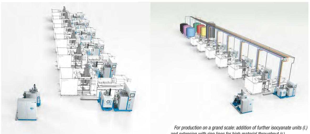
*For production on a grand scale: addition of further isocyanate units (l.)
