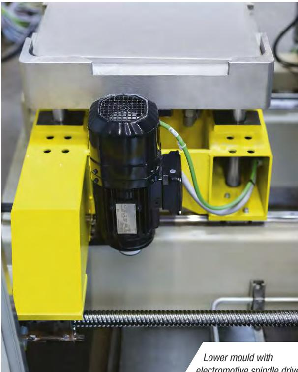
Lower mould with electromotive spindle drive
