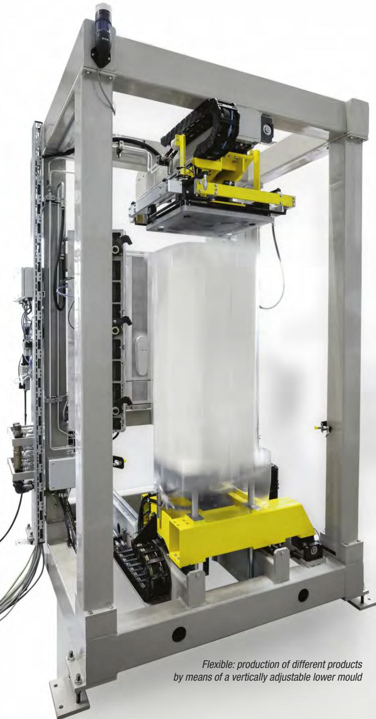
*Flexible: production of different products by means of a vertically adjustable lower mould*
