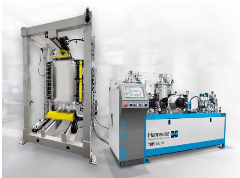
New mould carrier concept: a clamping device moves the foamed part completely out of the mould for easy removal. A TOPLINE high-pressure metering machine of size 650/650 assumes the metering task in the plant network.
