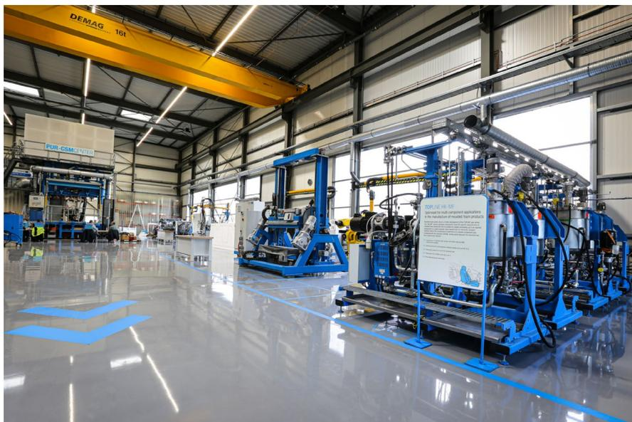
Better utilization and shorter distances within the approximately 1000 square meter hall. In the foreground: 6-component high-pressure metering machine with 40 ton mold carrier.
